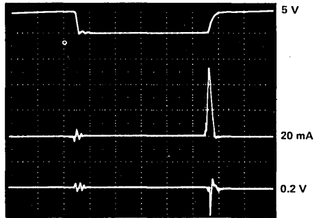
l) SN74ALS1000A load: C_L = 50 \text{ pF}
