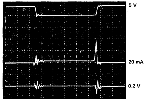
b) SN74S00 load: C_L = 50 \text{ pF}
