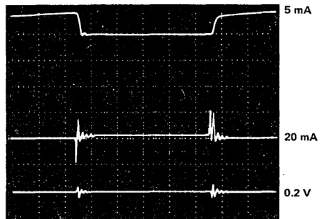
d) SN74LS00 load: C_L = 50 \text{ pF}
