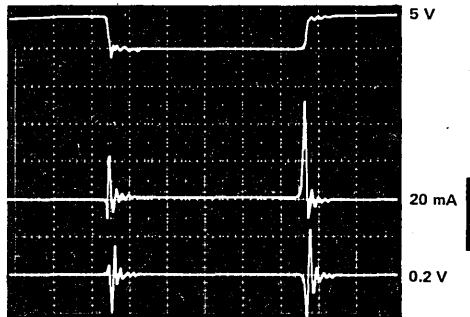
f) SN74AS00 load: C_L = 50 \text{ pF}
